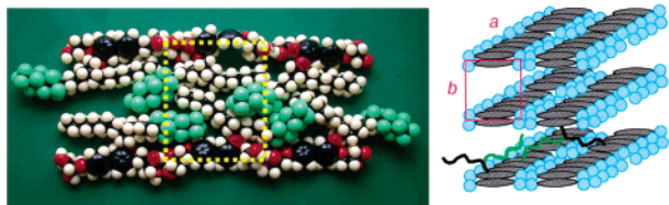
Figure 5. Proposed model of the organization of compound 2 in the columnar mesophase \text{Col}_r ( p2mm ). Due to the positional correlation between the layers and the additional electron density modulation within the lipophilic sublayers, an in-plane periodicity in a -direction can be found in the diffraction pattern of 2 which cannot be detected for the \text{LamA} phase of 1 . 8
